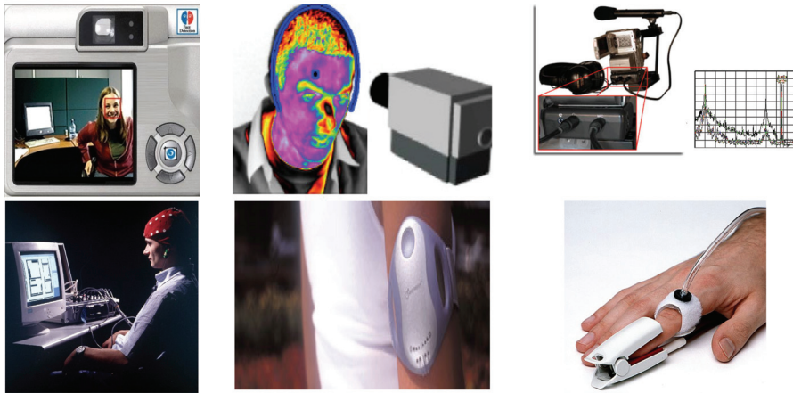
Figure 3: Examples of sensors used in multimodal affective data acquisition: (a) camera for visible imagery, (b) microphone(s) for audio recording, (c) infrared camera for thermal infrared (IR) imagery, (d) body media sense wear for physiological signal recording, (e) pulse wave signal recorder clipped on the finger, and (f) electroencephalogram (EEG) for brain/scalp signals recording and measurement.
