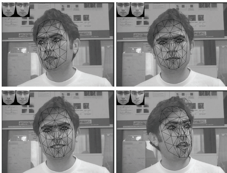
Figure 13: Simultaneous tracking and recognition associated with a 600-frame video sequence depicting non- frontal head poses.
